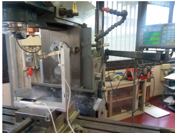
Figure 4. The mill equipped with the three axes movement system. The stick (a) was fixed to the static structure of the mill also hosting the mill tool (b). The VG structure (c) was secured by a grip to the three axes moving block of the mill (d), controlled numerically. The stick was used both to measure the LEAPs position with respect to the mill reference system and to collect spatial measurements inside the ROI.
