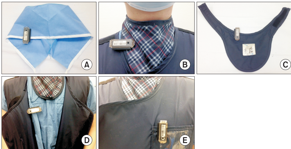
Fig. 2. Thermoluminescent dosimeters were placed on the forehead (A), outside the thyroid protector (B), inside the thyroid protector (C), inside the apron (D), and outside the apron (E).
