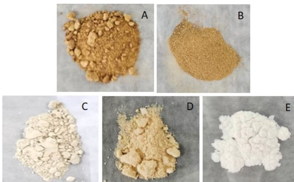
Figure 2. The images of IHRPs purified by different methods: (A) sewage method; (B) 500 Da membrane filtration; (C) column chromatography; (D) 4% activated carbon adsorption; (E) 8% activated carbon adsorption.
