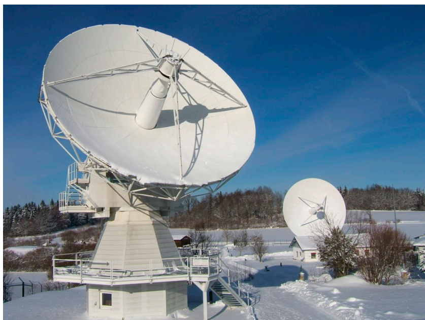
Figure 1. Photograph of the new 13.2 m diameter TTW1 radio telescope (left, foreground) and the 20 m diameter RTW (right, background) at the Geodetic Observatory Wettzell, Germany.
