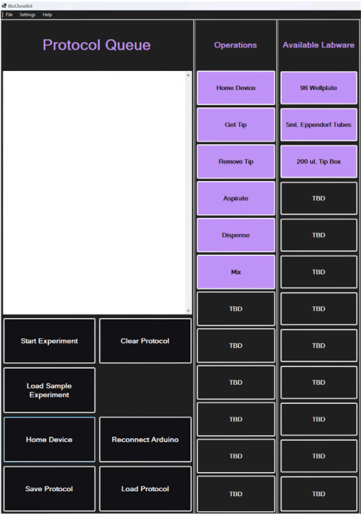
Fig. 5. The left side of the front-end includes the Protocol Queue which displays the selected operations in order. Also included are the potential Operations and Available Labware. Underneath the Protocol Queue are buttons used to control the software such as Start Experiment, Clear Protocol, Load Sample Experiment, and more.
