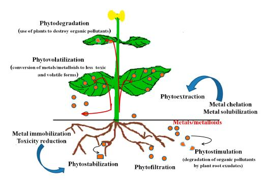
Figure 3. Processes used in phytoremediation of heavy metals.
