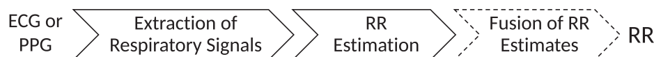
Figure 2. The three stages of a respiratory rate (RR) algorithm, which estimates RR from either the ECG or the PPG. The dashed stage is optional. Adapted from Pimentel et al (2015).
