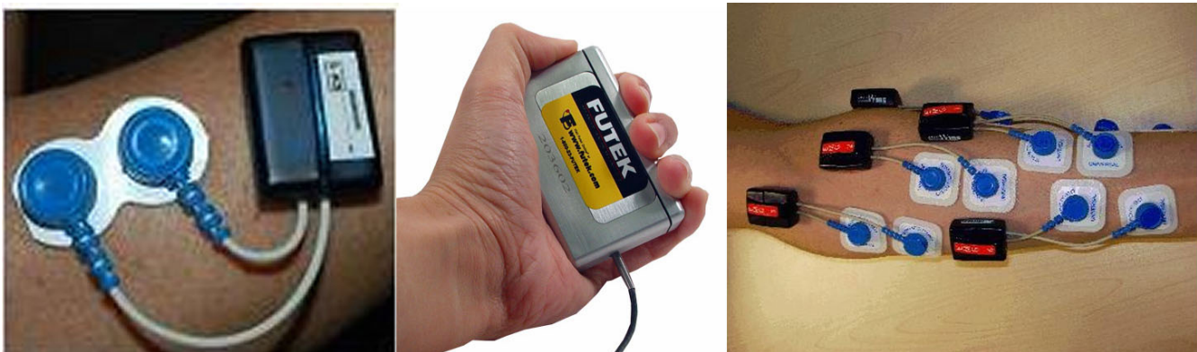
Figure 2 Part of the experimental setup: (left) an EMG wireless electrode; (center) the force sensor; (right) typical placement of the EMG electrodes on a subject's forearm (ventral side).
