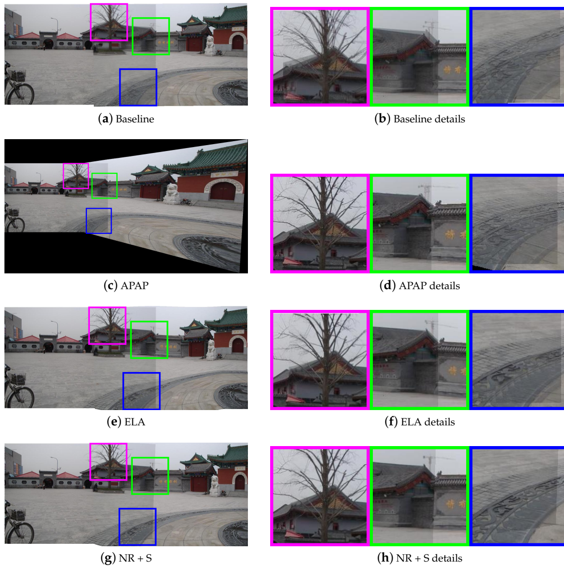
Figure 7. Comparison of stitching quality on “temple”. (a,b) are results of the baseline with obvious local misalignments. (c,d) are results of as-projective-as-possible (APAP). (e,f) are results of elastic local alignment (ELA). (g,h) are results of nonrigid + similarity warping.
