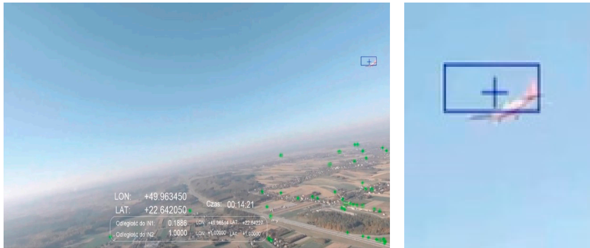
Figure 8. Scenario related to Figure 5A; afternoon, sun ~120 degrees to the left, altitude ~300 m; distance to intruder: 188 m.
