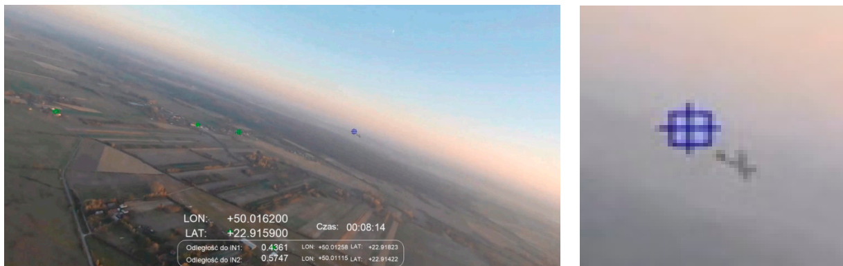
Figure 9. Scenario related to Figure 5C; evening, sun ~90 degrees to the right, altitude ~200 m; distance to intruder: 436 m.
