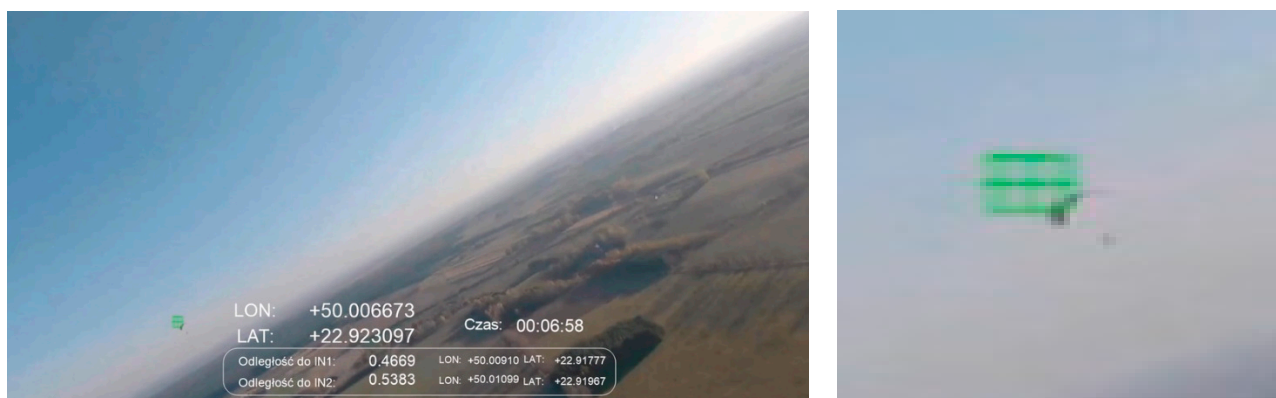
Figure 13. Detection of paraglider; afternoon, sun ~90 degrees to the right, altitude ~150 m, distance to intruder: 466 m.
