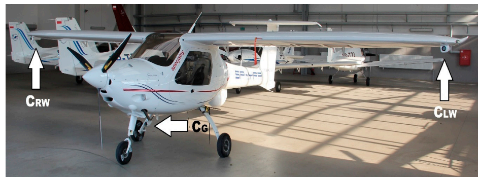
Figure 3. General view of the Czajka MP-02 airplane with an indication of the location of the observation sensors ( C_{RW} —right wing camera, C_{LW} —left wing camera, C_G —camera installed on the chassis).
