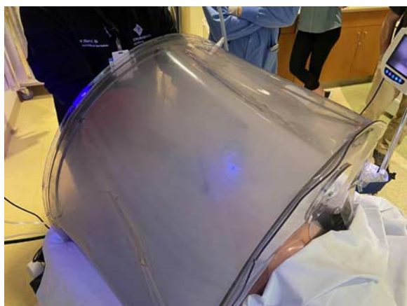
FIGURE 4. Aerosol containment in fogger testing.
