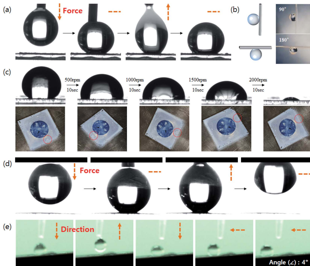
Fig. 4 (a) Dropping water droplet and its movement on a sticky structured coating using SPRCSPs (15 g VDF). (b) Water droplet behavior at 90° and 180° inclination of the sticky SPRCSP coating (VDF 15 g). (c) Water droplet behavior on the sticky SPRCSP coating (VDF 15 g) after applying a rotational force while gradually increasing the rotational speed (500–2000 rpm) for 10 s. (d) Dropping water droplet and its and movement on a low-strength sticky SPRCSP coating (VDF 18 g). (e) Images of the moving water droplet on a SPRCSP coating (VDF 18 g) with a tilting angle of 4°.
