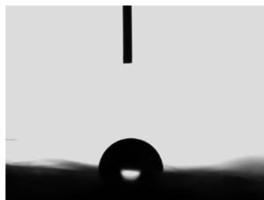
Figure 5. Static contact angle between distilled water and the M. floridulus fiber.
