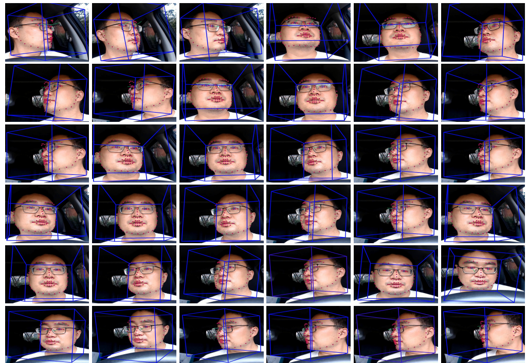
Figure 4. The driver status extraction results of all the partitioned gaze zone. The first row shows the results of GZ1~GZ6. The second row shows the results of GZ7~GZ12. The third row shows the results of GZ13~GZ18. The fourth row shows the results of GZ19~GZ24. The fifth row shows the results of GZ25~GZ30. The last row shows the results of GZ31~GZ36. GZ: Gaze Zone.
