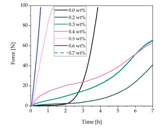
**Figure 4.** Results of a penetration test (MILD—multipurpose incremental loading device) of CEM I with different dosages of superplasticizer (w/c = 0.36).
