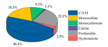
Figure 3. Composition of the hardened CEM I after an infinite duration of hydration (w/c = 0.36).
