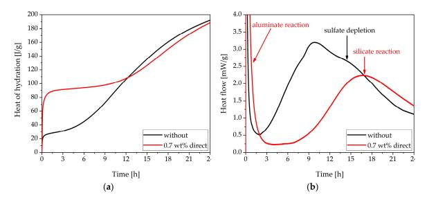
**Figure 5.** Calorimetric results of CEM I without superplasticizer (SP) and with direct addition of 0.7 wt% of SP (w/c = 0.36): (a) Heat of hydration and (b) Heat flow.
