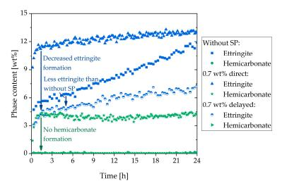
**Figure 16.** Ettringite and hemicarbonate content of the sample without SP, with direct addition of 0.7 wt% of SP, and with a delayed addition.
