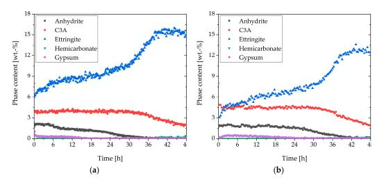
**Figure 8.** Phase development of the aluminum-containing phases of CEM I during 48 h of hydration (w/c = 0.36) with: (a) 2 wt% of gypsum and 0.7 wt% of SP (direct addition), and (b) 0.7 wt% of SP (delayed addition).
