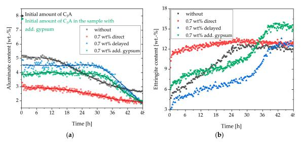
**Figure 10.** Summary of the (**a**) aluminate and (**b**) ettringite content of the samples without SP, with direct addition of 0.7 wt% of SP, with a delayed addition of 0.7 wt% of SP, with 2 wt% of additional gypsum, and direct addition of 0.7 wt% of SP.
