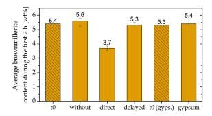
**Figure 9.** Average brownmillerite content during the first 2 h at the beginning of hydration ( $t_0$ ), without SP, with direct addition of 0.7 wt% of SP, with a delayed addition of 0.7 wt% of SP, and with 2 wt% additional gypsum and direct addition of 0.7 wt% of SP.
