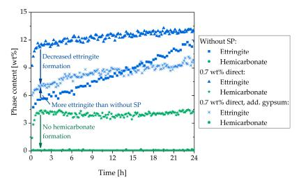
**Figure 15.** Ettringite and hemicarbonate content of the sample without SP, with direct addition of 0.7 wt% of SP, and with additional gypsum and direct addition of 0.7 wt% of SP.
