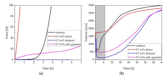
**Figure 7.** Comparison of the rheological behavior of a sample without SP, with 0.7 wt% of SP (direct addition), 0.7 wt% of SP (delayed addition), and 0.7 wt% of SP (direct addition), and with an additional amount of 2 wt% of gypsum measured with (**a**) a penetration test (MILD), (**b**) ultrasound velocity.
