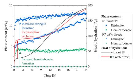
**Figure 14.** Ettringite and hemicarbonate content of the sample without SP and with direct addition of 0.7 wt% of SP and the heat evolution of both samples.
