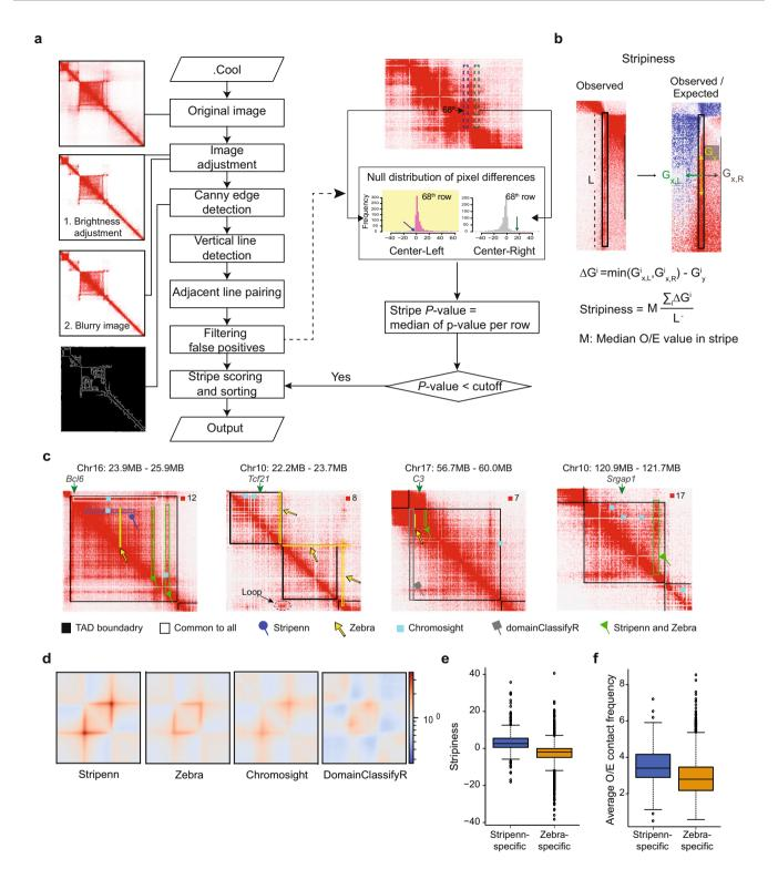
than 10 pixels are connected to the diagonal line. Canny edge detection predicts two edges for each stripe and adjacent lines within a pre-defined distance are paired, forming a single vertical stripe. Together, Stripenn adapts principles from digital image processing and edge detection techniques to demarcate architectural stripes.
