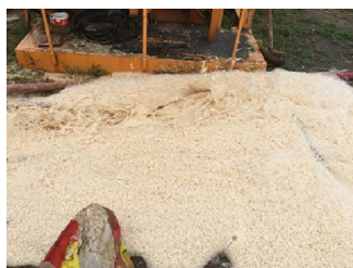
Figure 17. On-site perfusion of the three-phase foam.
