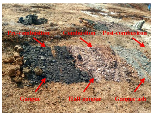
Figure 13. Burning state of coal gangue.
