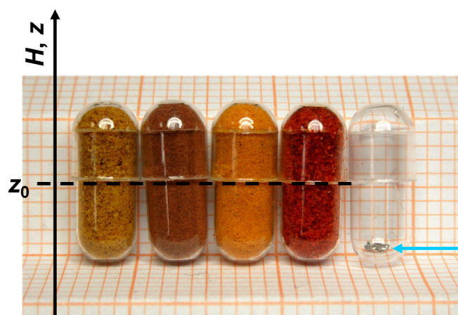
Figure 3. Some examples of the use of small capsules (#5 in this example) for measurements of substances that otherwise would be difficult to reliably and cleanly mount in the SQUID sample chamber. From the left, the first four are fully loaded, so no alignment problems are expected. The magnetic “center of gravity”, marked by the dashed black line, coincides with that of the capsules. These capsules house common curry, cinnamon, turmeric, and red pepper powders. The fifth capsule houses a small, 2.1 mg, crystallite of SnTe, used later to validate the in situ compensation method put forward in this report. As indicated, the crystallite sitting at the bottom of the capsule, is shifted by about 5 mm from the center of the capsule, causing serious experimental errors due to alignment problems, discussed in this section.
