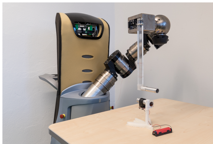
Figure 6. Experimental set-up for evaluation of spatial sensor resolution.
