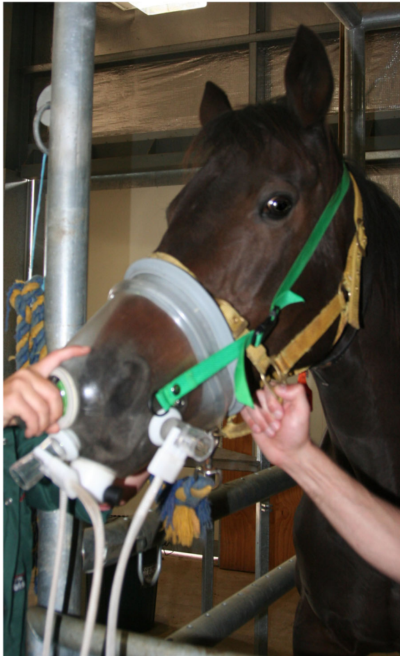
Fig. 1 Facemask in position with three bi-directional pitot flow meters attached. Flow data was collected simultaneously from each sensor and summed to provide volume and flow results. Gas analysis was performed on samples aspirated continuously from the middle sensor. The horse's head was maintained in the position shown throughout testing
