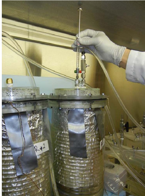
Fig. 6. 22 week-long trial of anaerobic poultry carcass disposal in 6 L reactors: collection of biogas samples.
