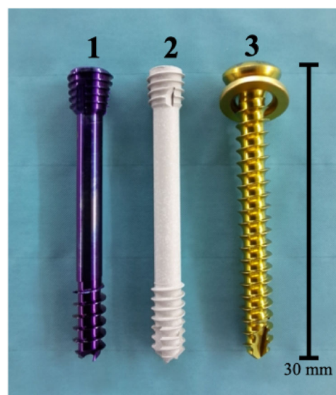
FIGURE 1 The used implants for refixation of the solid posterior cruciate avulsion Fragment, where differences between screw designs can be seen. (1) Titanium headless compression screw ( 3.5\text{ mm} \times 30\text{ mm} , partially threaded CCHS, Synthes). (2) Magnesium-based headless compression screw ( 3.5\text{ mm} \times 30\text{ mm} , partially threaded mm.CS, Medical Magnesium). (3) Titanium cortical screw fixation ( 3.5\text{ mm} \times 30\text{ mm} fully threaded + titanium washer, Synthes).
