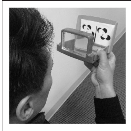
Figure 5. The stereogram viewer used for clay modeling.
