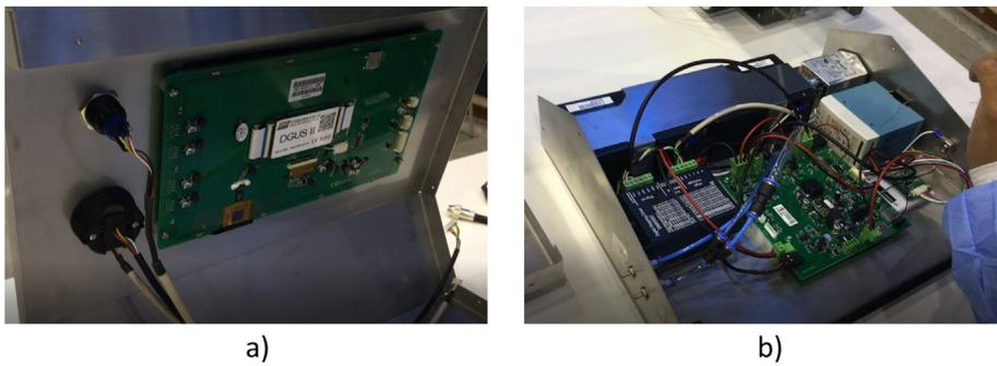
Fig. 8. (a) Touch screen and interface buttons (b) Control and power boards.
