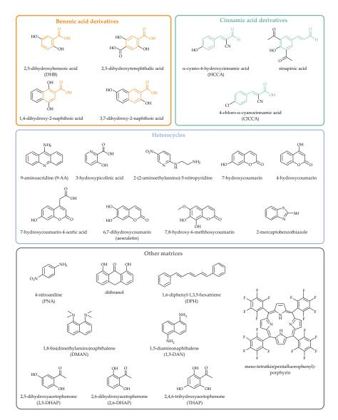
**Figure 2.** Chemical structures of the organic MALDI matrices which will be explicitly mentioned in this review. The backbones of both benzoic acid (orange) and cinnamic acid (green) derivatives are highlighted. Please note that this is only a small selection and many other compounds were also found to be useful MALDI matrices.
