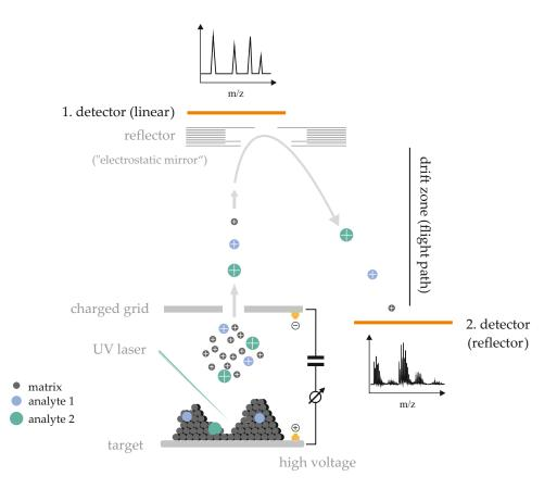
**Figure 1.** Simplified schema of the positive ionization matrix-assisted laser desorption/ionization-timeof-flight (MALDI-TOF) process occurring in the mass spectrometer (for details see text and Reference [18]). The influence of the detection using either the linear or the reflector mode is emphasized in the figure.
