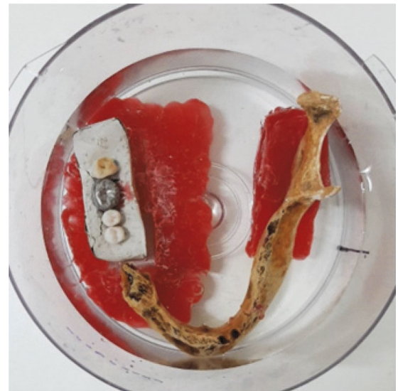
Fig. 3. Phantom placed in a plastic container filled with water to simulate soft tissue and with a partial dry mandible to simulate the opposite side.
