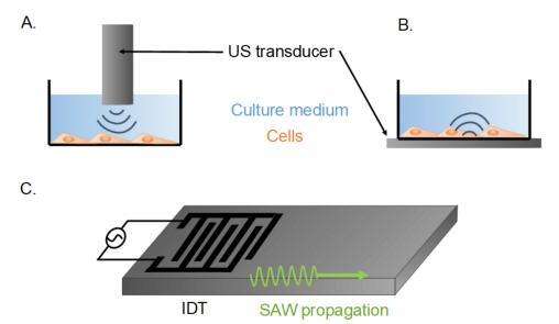
**Figure 1.** Schematic view of cell-stimulation systems of low- or high-intensity ultrasound stimulation. (**A**): Cells stimulated mainly by the shear flow induced by a US transducer immersed in the culture well. (**B**): Cells stimulated mainly by the mechanical vibrations of the culture well. US stimulated by the US transducer under it. (**C**): Piezo-electric system with an interdigital transducer (IDT) inducing surface acoustic waves (SAW).
