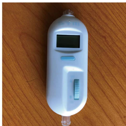
Fig. 4 Measurement of the intraluminal balloon pressure. a The mini electronic pressure transducer for intraluminal balloon pressure recording. b The effect of contrast volume on the intraluminal balloon pressure in vitro
