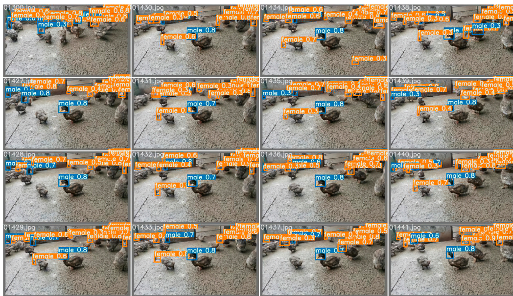
Figure 16. The sample results of scheme two. The locations, masking conditions, and individual behaviors of the ducks vary in each extracted frame. Change to the training dataset reduces the number of additional noise points and slightly improves the success of duck detection and the accuracy of gender estimation, but the accuracy is still not high.
