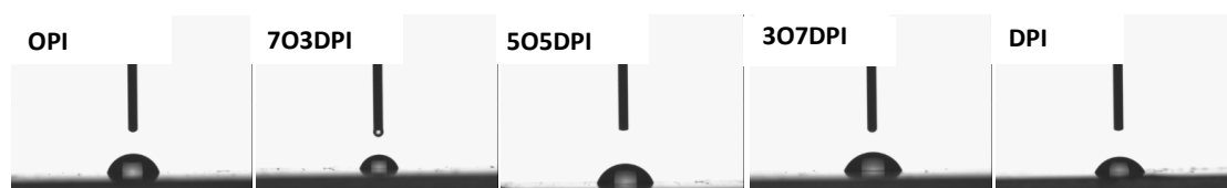
Figure 5. Images of water contact angle test of polyimide films.
