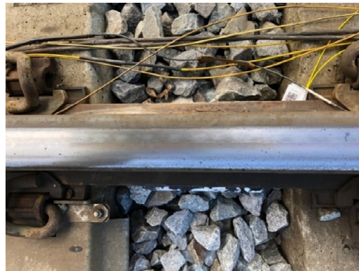
Figure 7. Picture of the setup: pad installed under the rail.
