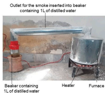
Figure 1. Preparation of plant-derived smoke solution. Plant material is burnt in the specified chamber through an electric heater. The smoke coming from burning plant material is collected through a pipe by bubbling this smoke into 1 L distilled water at the other end of pipe. All the setup is completely sealed to avoid any smoke escape.
