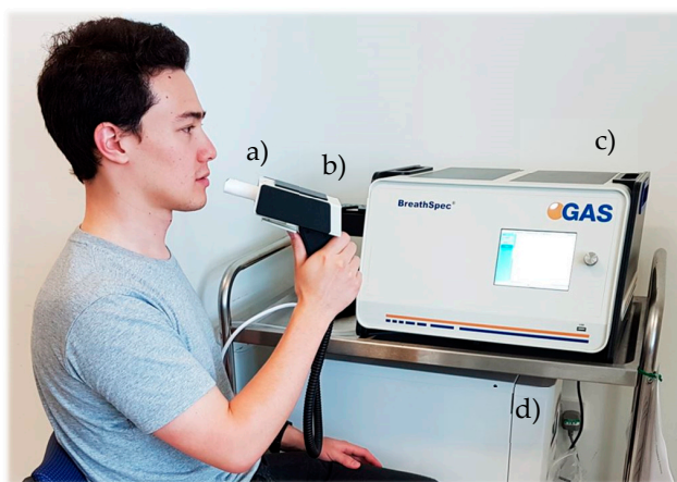
Figure 4. G.A.S. BreathSpec GC-IMS: (a) Plastic disposable mouthpiece; (b) Mouthpiece holder; (c) GC-IMS instrument; (d) Nitrogen generator.
