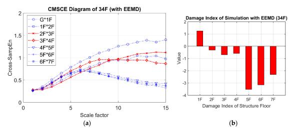
**Figure 14.** (a) CMSCE diagram of damage on the third and the fourth floor (34F) with EEMD; (b) Damage index of damage on the third and the fourth floor with EEMD.
