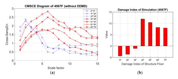
**Figure 11.** (**a**) CMSCE diagram of damage from the fourth to the seventh floor (4567F); (**b**) Damage index of damage from the fourth to the seventh floor.
