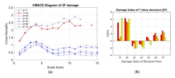
**Figure 21.** (a) The experimental CMSCE diagram of damage on the second floor (2F); (b) Damage index of damage on the second floor.
