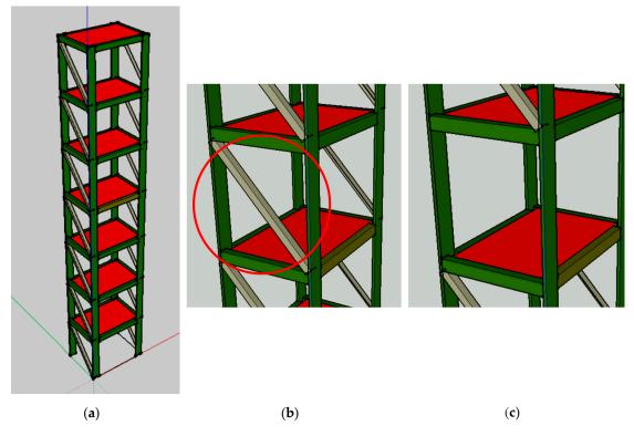
Figure 5. (a) View of the numerical model. (b) The undamaged scenario. (c) The damaged scenario.
