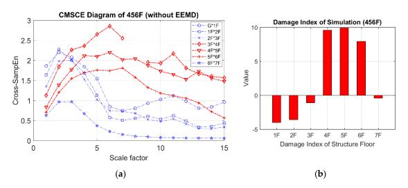
**Figure 10.** (**a**) CMSCE diagram of damage from the fourth to the sixth floor (456F); (**b**) Damage index of damage from the fourth to the sixth floor.
