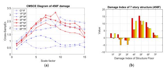
**Figure 23.** (**a**) The experimental CMSCE diagram of damage from the fourth to the sixth floor (456F); (**b**) Damage index of damage from the fourth to the sixth floor.
