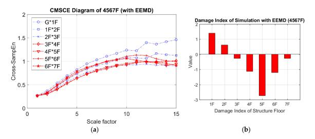
**Figure 16.** (**a**) CMSCE diagram of damage from the fourth to the seventh floor (4567F) with EEMD; (**b**) Damage index of damage from the fourth to the seventh floor with EEMD.
