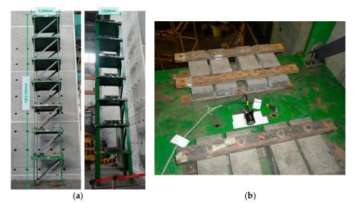
Figure 17. (a) A seven-story scale-down benchmark structure; (b) The arrangement of velocity meter and mass block.
