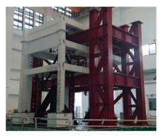
Figure 2. Three-story RC structure.
