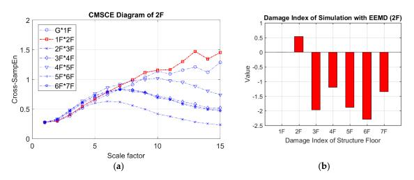
**Figure 13.** (a) CMSCE diagram of damage on the second floor (2F) with EEMD; (b) Damage index of damage on the second floor with EEMD.
