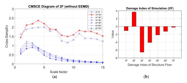
**Figure 8.** (a) CMSCE diagram of damage on the second floor (2F); (b) Damage index of damage on the second floor.
