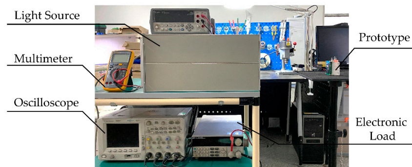
Figure 5. Photos of testing platform for the hybrid power system.
