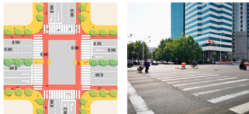
Figure 20. Setting Up a Safety Island at the Intersection of Shiyijing Road and Bawei Road.
