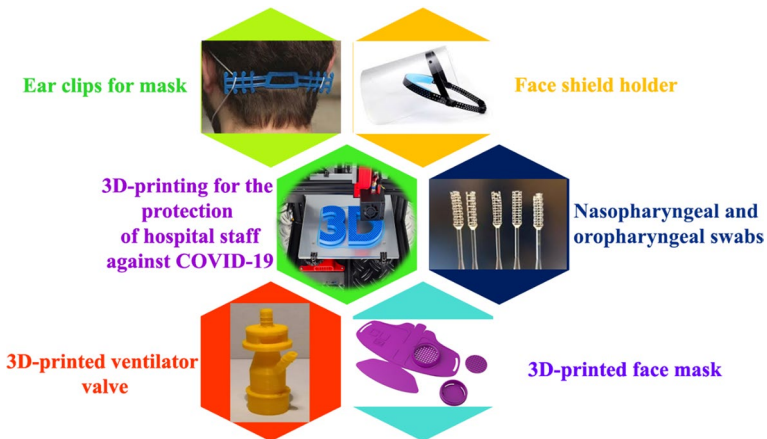
Fig. 8 Different equipment uses in COVID-19 pandemic produced by 3D printing
