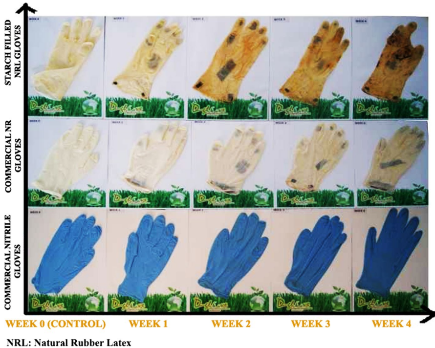
Fig. 4 Effect of biodegradation on Biodegradable Gloves (starch-filled NRL gloves), Commercial NRL gloves and Commercial Synthetic NBR gloves [12]
