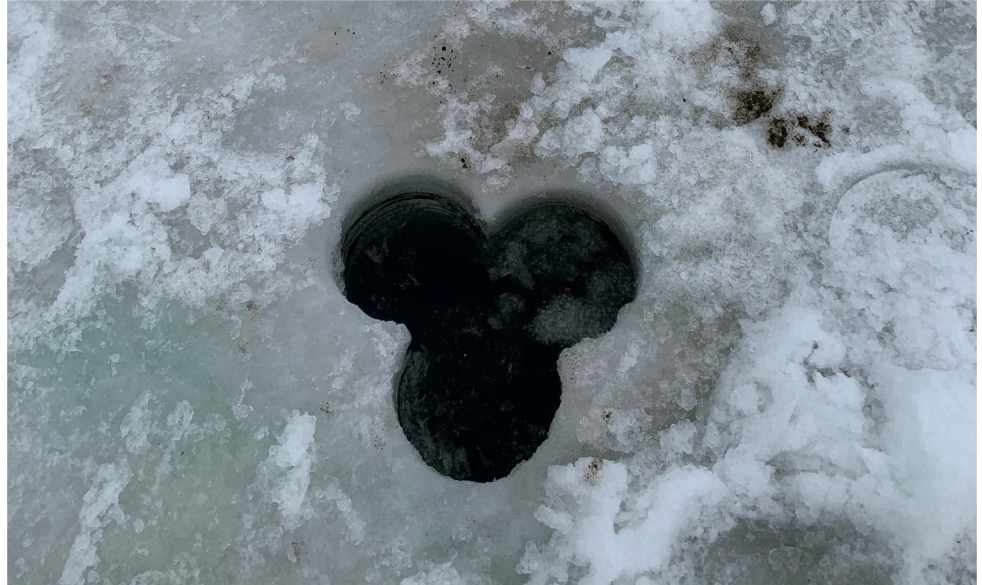
Fig 2. Holes for through-ice sampling. Image of the hole pattern drilled with ice auger to create large enough holes to accommodate D-net and scooping motions used in sediment sample collection.
