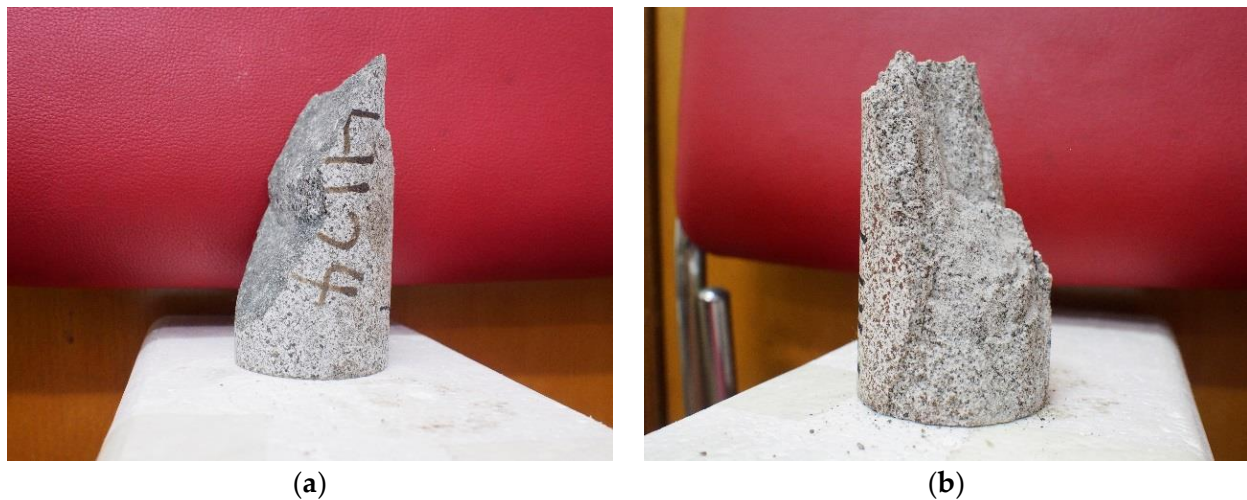
Figure 3. Granite specimens after uniaxial compression tests subjected to heat treatment at (a) 200 °C and (b) 1000 °C.
