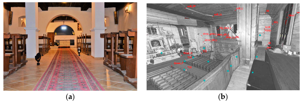
Figure 5. Measurement targets in the underground chapel (a) and the view of the scanning data in the reflectance intensity of the laser beam—one of the scanner positions inside the church (b).
