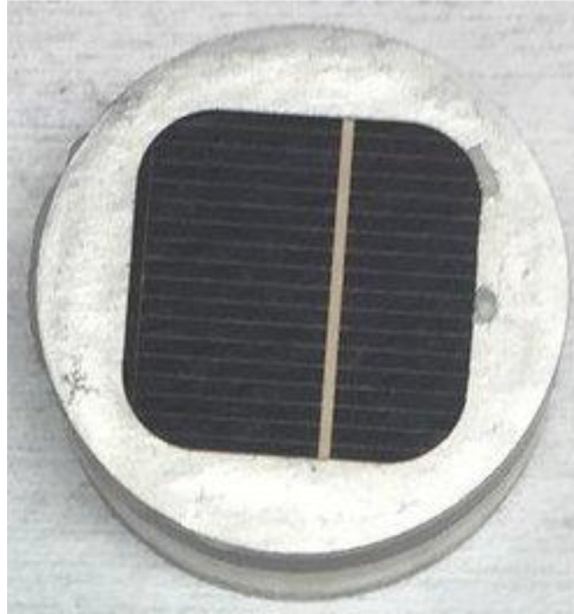
Fig. 1. Photograph of a 25 mm x 25 mm mc-Si solar cell sample mounted for grinding and polishing.
