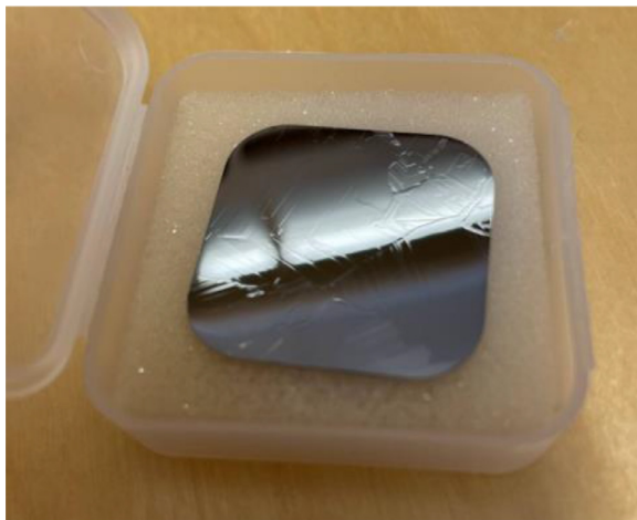
Fig. 4. A photograph of a sample after the final CMP step.
