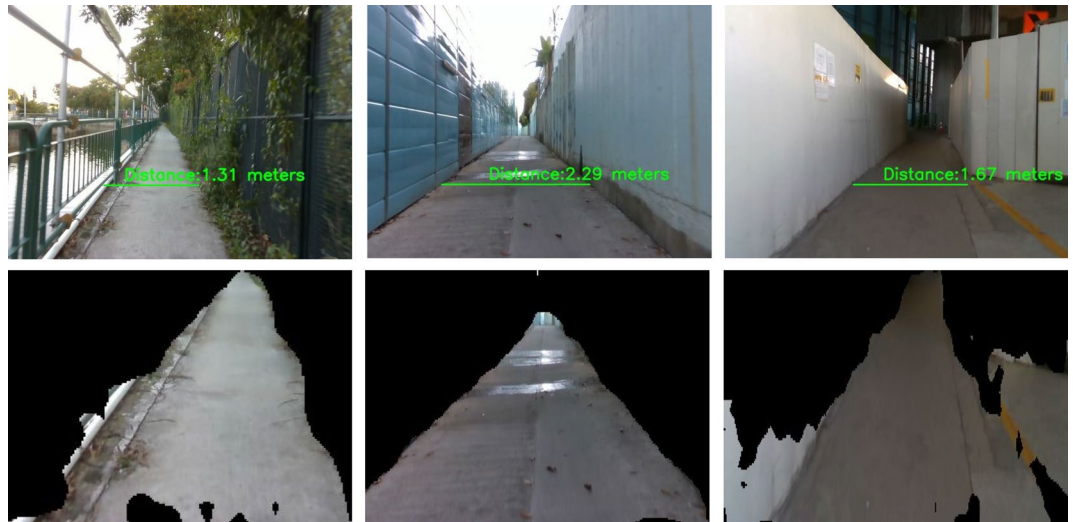
Figure 29. Offline results: pavement width estimation from pavement segmented region.
