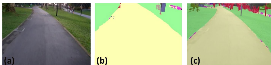
Figure 34. DeepLabv3+ segmentation results: pavement with night mode.
