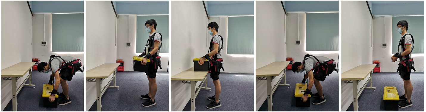
Fig 3. A subject performing the whole lifting process with the exoskeleton. The toolbox was set at 20% MVE of the subject and the table had been adjusted to the waist height.
