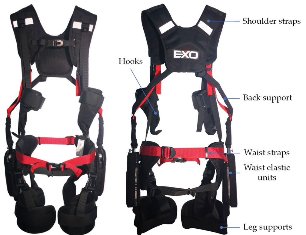
Fig 1. The structure diagram of IPAE used in the tests. It consists of a back support, waist elastic units, leg supports, hooks, shoulder straps and waist straps showed in two views: (a) front view; (b) rearview.
