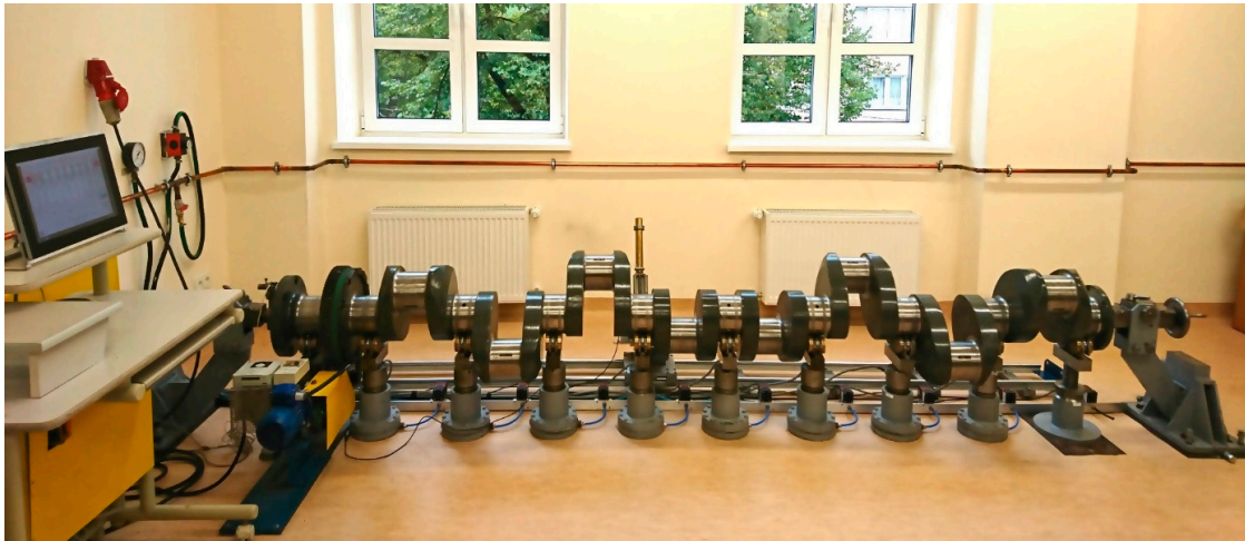
Figure 18. A prototype test bench developed at the Maritime University in Szczecin for the measurement of the geometric deviation in large-size crankshafts equipped with a flexible support system.
