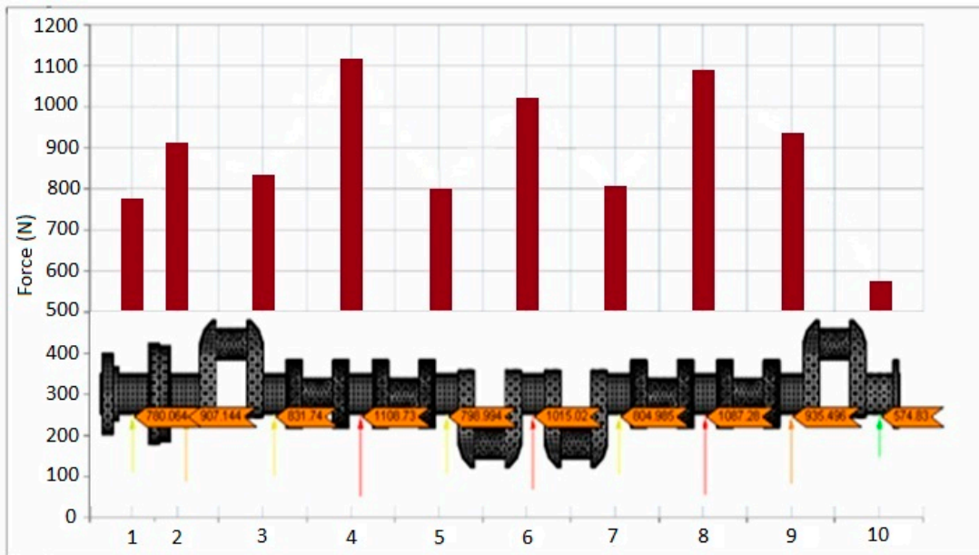
Figure 2. Distribution of forces ensuring zero deformation of the main journal of the crankshaft of a Buckau Wolf R8DV 136 engine for a shaft position of 0 °CA.
