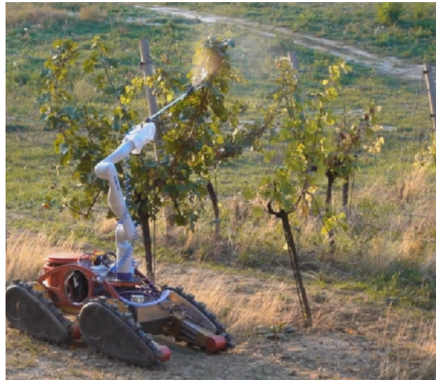
Figure 3. An ATMM in a vineyard spraying scenario. Spraying nozzle is attached to the robot arm, and the arm motion controls its pose relative to the mobile base.
