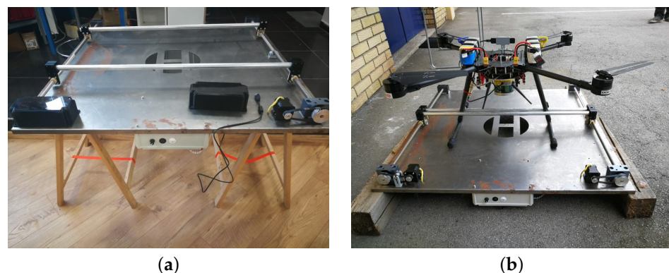
Figure 12. Test setups for the landing platform. (a) Test setup in the laboratory with a control box. (b) Outdoor test setup with manual landing of the LAAR and semi-automatic control of the LP in Zagreb, Croatia.
