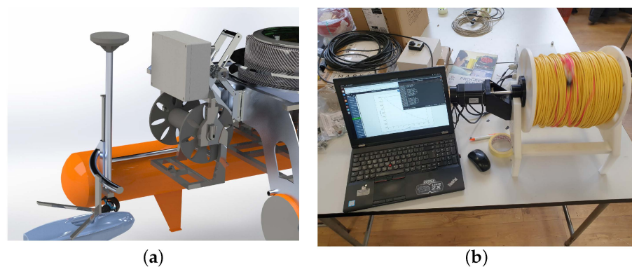
Figure 15. (a) SolidWorks model of the tether management system and docking station for the ROV aboard the ASV Korkyra. Side view of the assembly on the ASV. (b) Laboratory testing of the prototype TMS.
