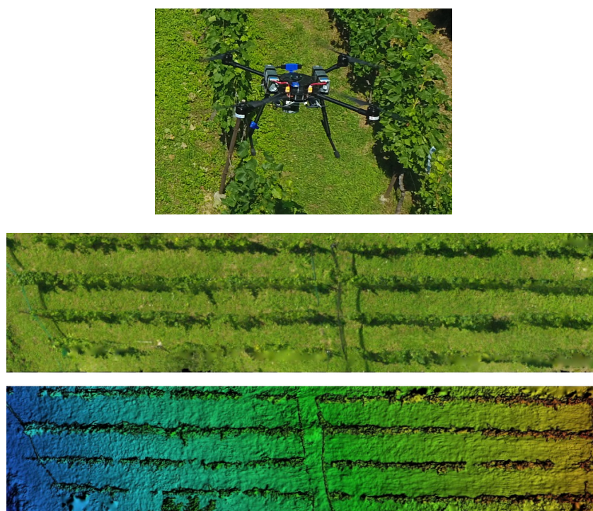
Figure 2. Monitoring the vineyard from the air, top —LAAR monitoring the vineyard, middle —stitched RGB image, bottom —generated 3D model.
