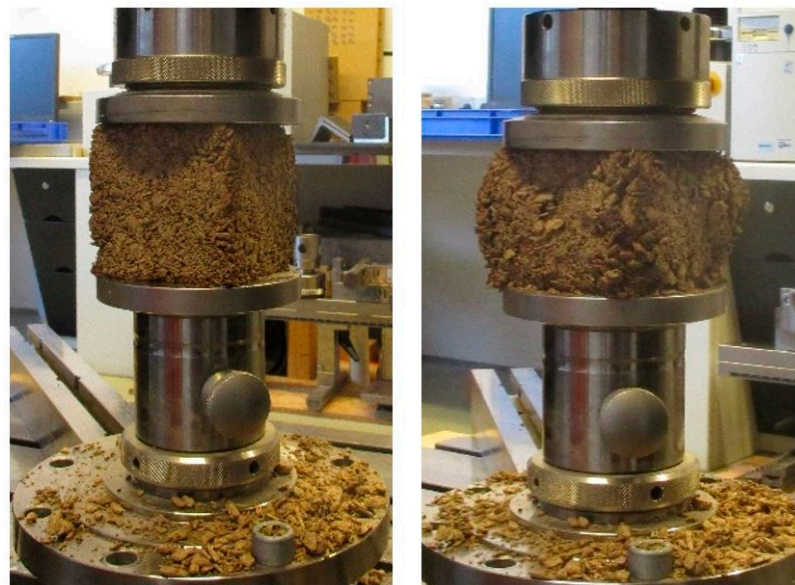
Figure 3. Compressive strength measurement at 10% compression of the 100 \times 100 \times 100 \text{ mm}^3 specimen using universal testing machine Zwick/Roell 250.
