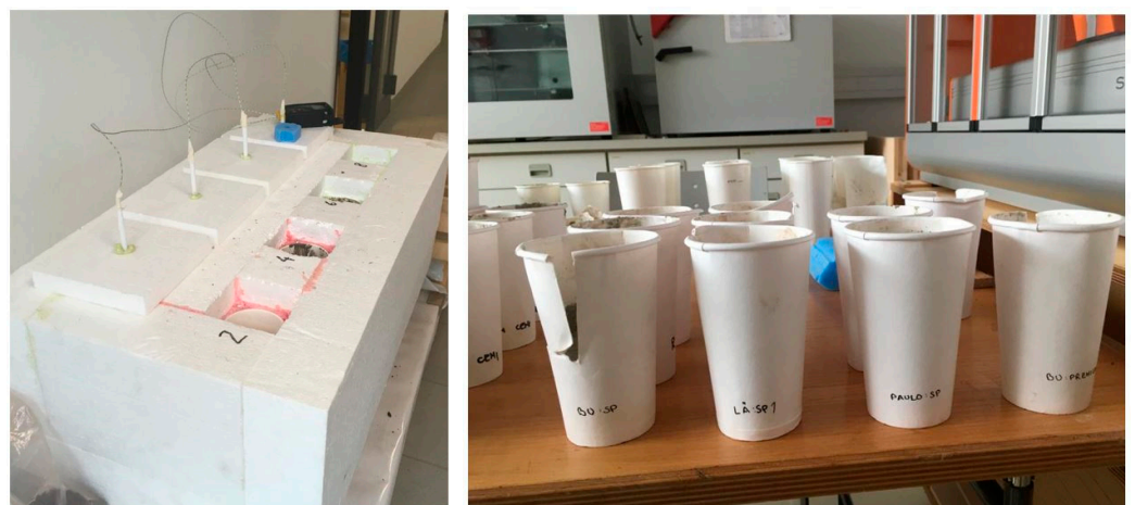
Figure 1. Insulation box (left) and paper cups with bark-cement mixture (right) for hydration temperature measurements.
