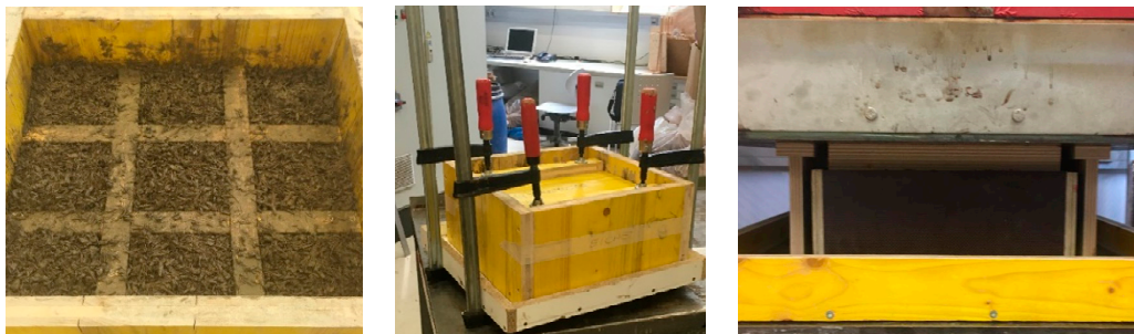
Figure 2. Test specimens of 100 \times 100 \times 100 \text{ mm}^3 in a forming frame (left); Compaction by screw clamps (middle) and compaction by hydraulic press (right).
