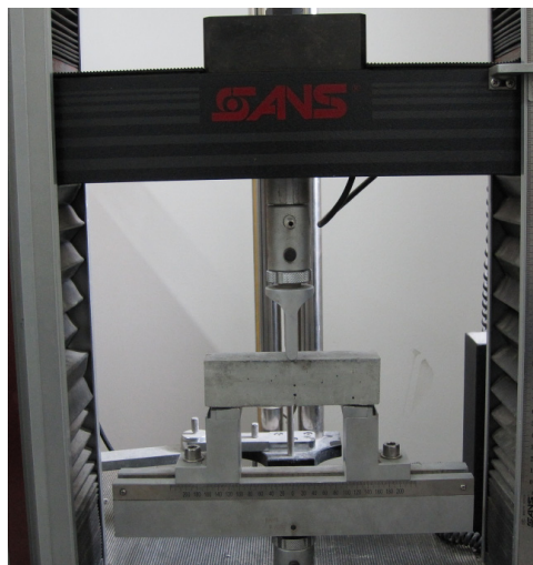
Figure 5. Three-point flexural loading setup.
