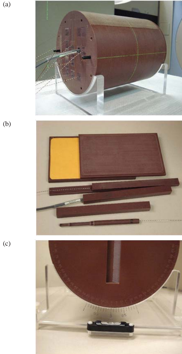
FIG. 1. IMRT Phantom: (a) phantom with multiple MOSFETs positioned for image guided dosimetry, (b) film, MOSFET and ion chamber holder, (c) phantom end plate showing angular scale.
