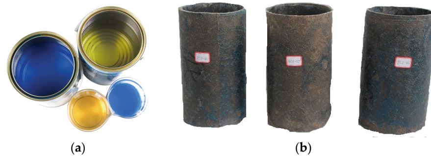
Figure 4. Production of JFRP tubes: (a) JN-C3P epoxy, (b) prefabricated JFRP tube.
