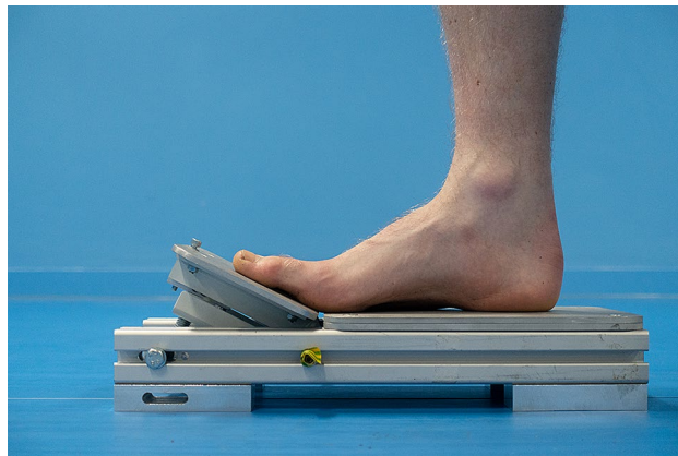
Figure 2. Image showing foot position on the dynamometer.
